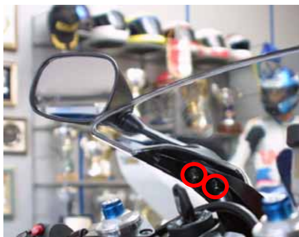
Figure 15: location of the left lateral mirror screws (inside view).
