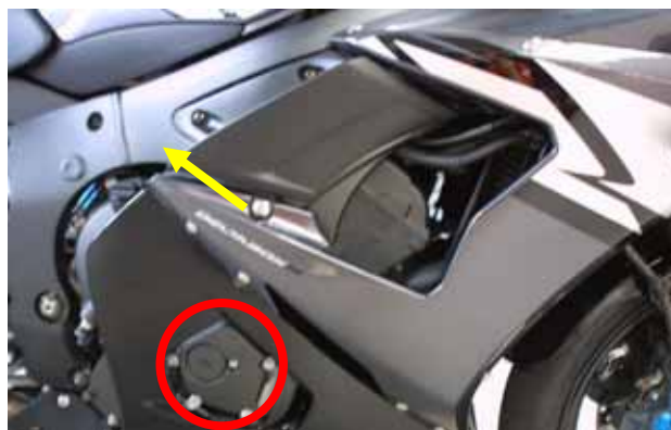
Figure 24: location of the on board speed connector
