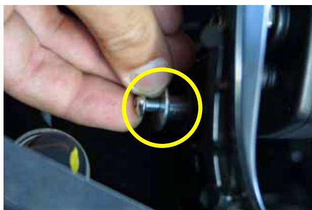
Figure 27: fixing MyChron 3 Plus / Gold to the bike.
