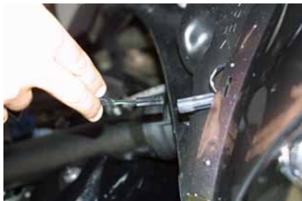
Figure 14: the turn signal connector.
