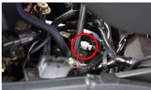
Figure 23: the on board speed connector.
