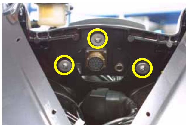
Figure 28: MyChron 3 correctly installed (rear view)
