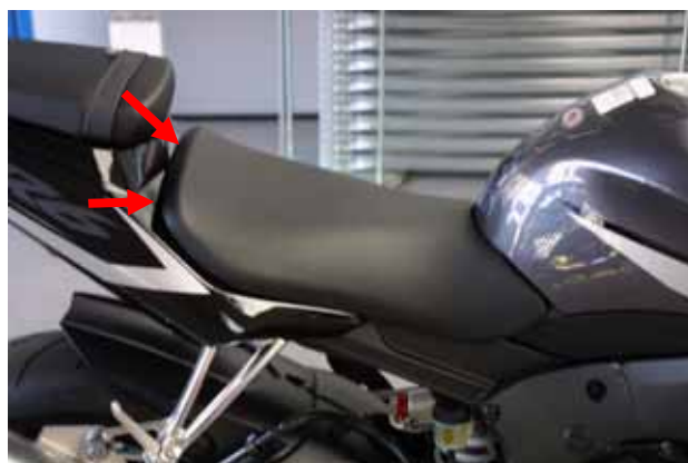
Figure 1: location of the seat screws.
