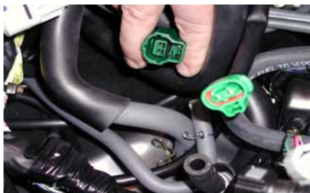
Figure 25: the on board water temperature connector
