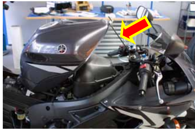
Figure 3:Uplifting the gas tank.
