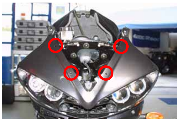
Figure 16: the front transparent fairing screws.
