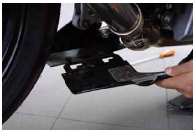
Figure 12: Slackening the groove of the lateral fairings
