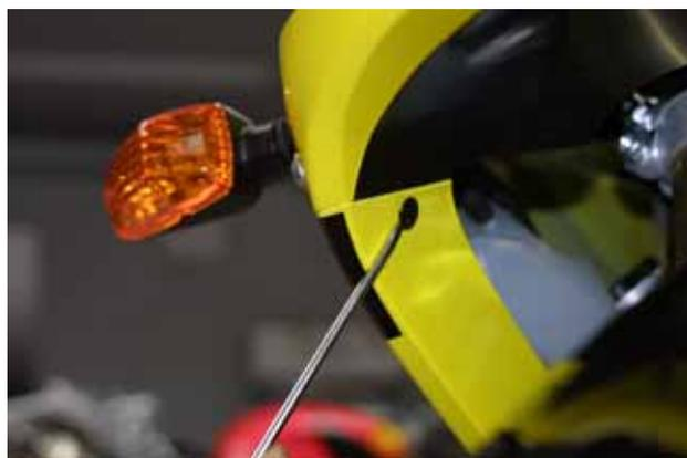
**Figure 7:** removing the plastic pin
