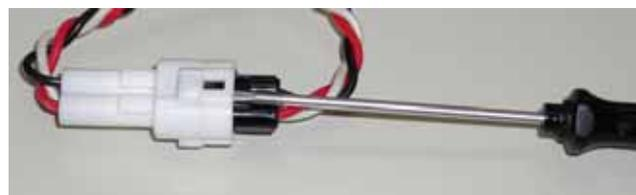
**Figure 20:** How to unplug a connector
