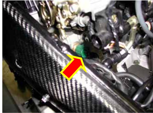
**Figure 19:** Water temperature connector – particular
