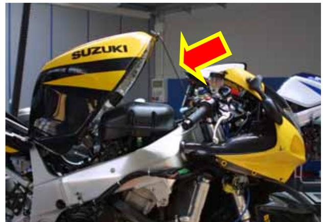
**Figure 11:** Uplifting the gas tank
