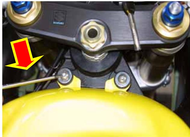
**Figure 10:** How to remove the gas tank
