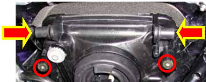
**Figure 29:** position of the 4 screws.
