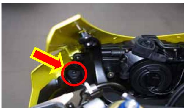
**Figure 12:** position of fairing and headlight screws
