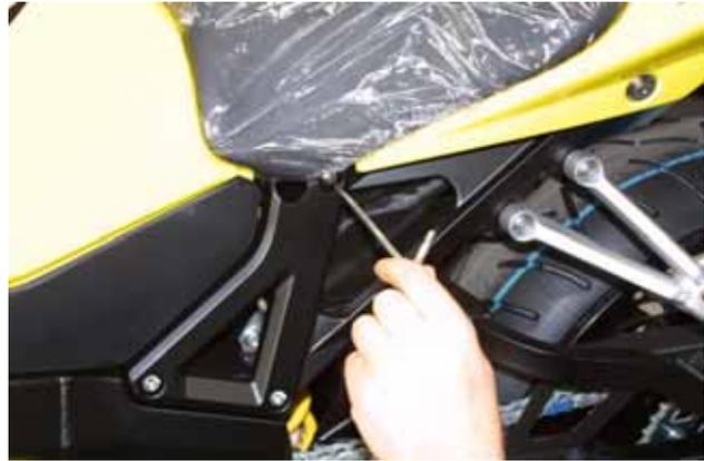
**Figure 9:** Unscrewing seats screw
