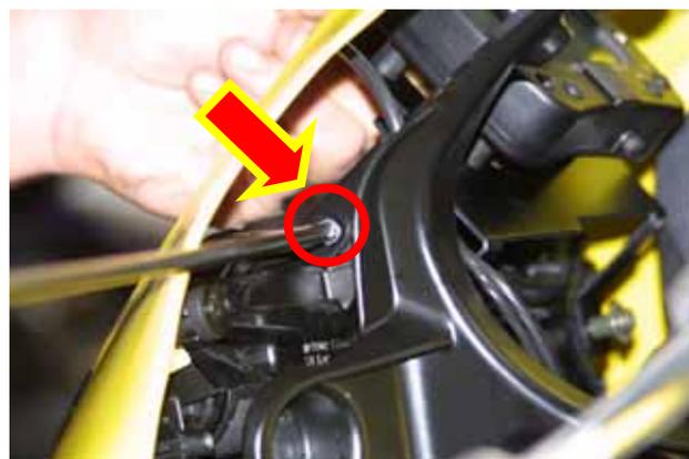
**Figure 30:** fixing the lateral screws
