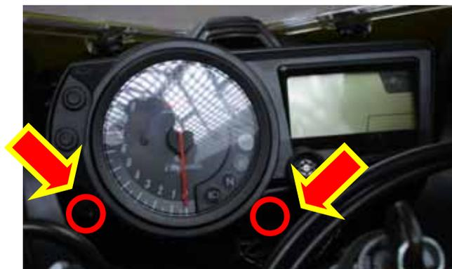
Figure 14: Position of the stock dash front screws.
