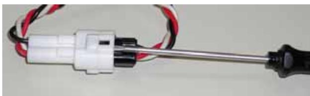
**Figure 20:** How to unplug a connector
