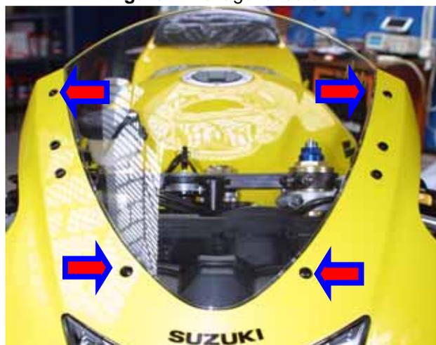
**Figure 3:** Front fairing – 4 Phillips recess screws.
