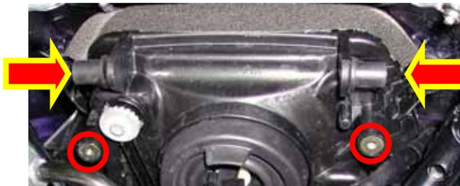
Figure 27: position of the 4 screws.
