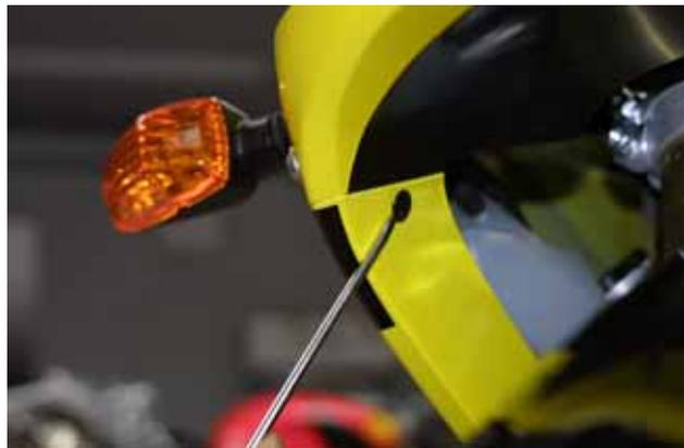
**Figure 7:** removing the plastic pin
