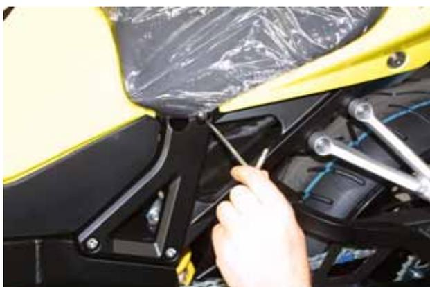
**Figure 9:** Unscrewing seats screw
