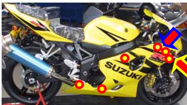
**Figure 4:** Right lateral fairing – screws/pins location
