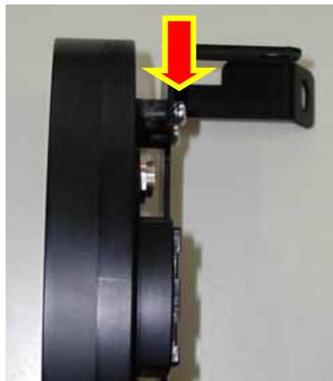
Figure 21: anti-vibration mountings – particular
