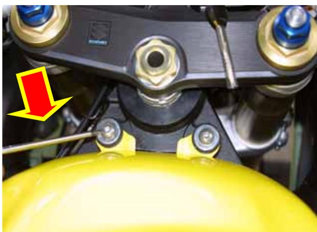
**Figure 10:** How to remove the gas tank
