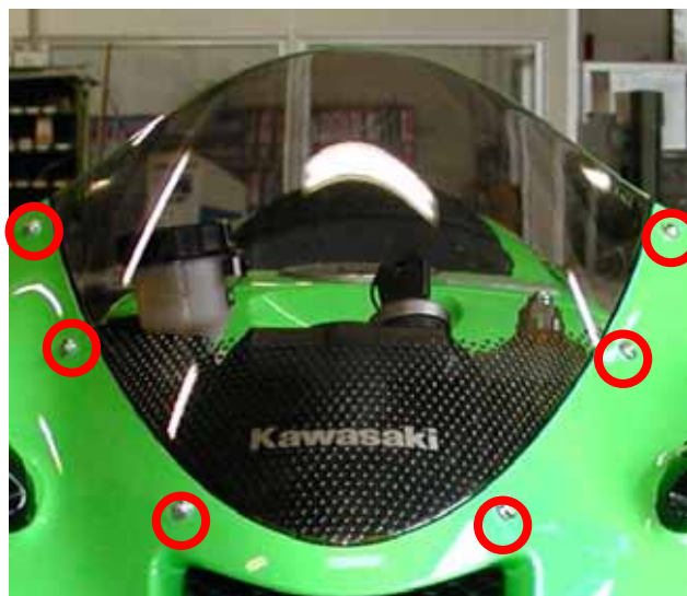
Figure 1: front transparent fairing – screws location
