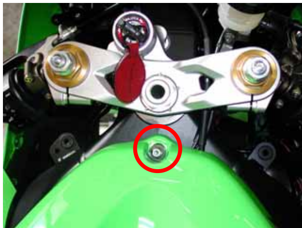
Figure 14: location of the gas tank screw
