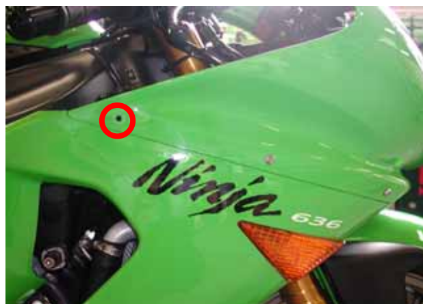
Figure 2: .Lateral screw to remove.
