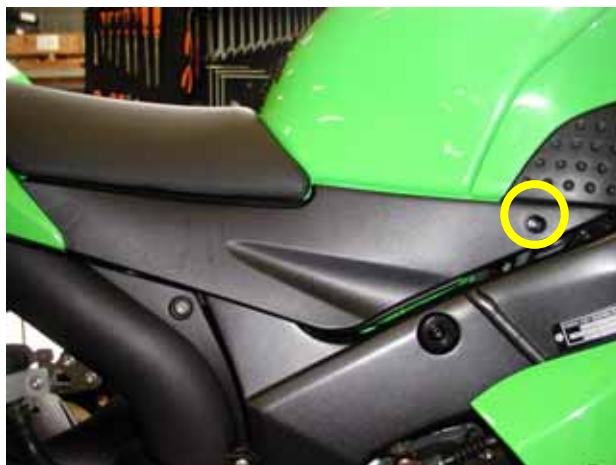
Figure 12: location of right plastic chassis screw
