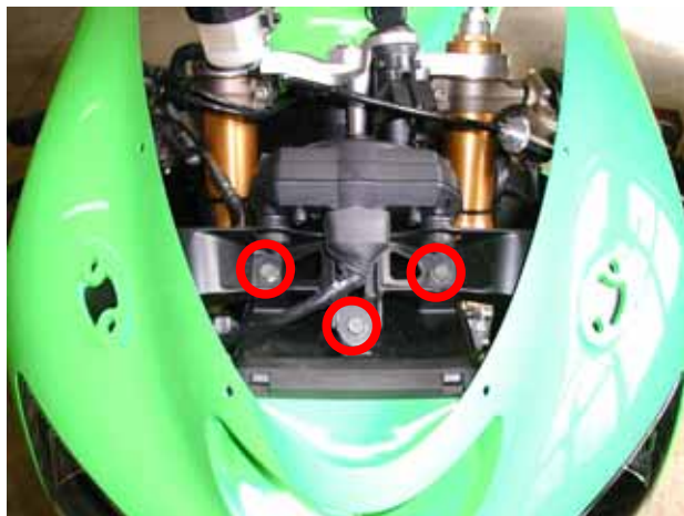
Figure 4: location of the little internal fairing screws
