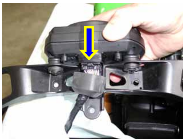
Figure 5: the on board wiring connector
