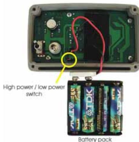
Figure 2: Infrared lap transmitter HIGH/LOW power switch
